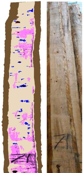
Scanned and photographed sample boards from surface defect scanning.
